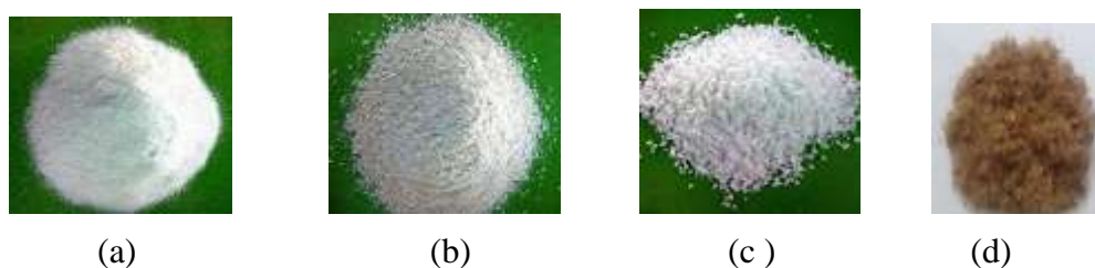
Figure 1 (a) Recycled polyethylene (b) polypropylene (c ) reused polystyrene and (d) betel nut shell fiber particles
